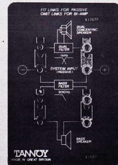
Terminal panel on FSM allows simple connection for bi-amp mode.
