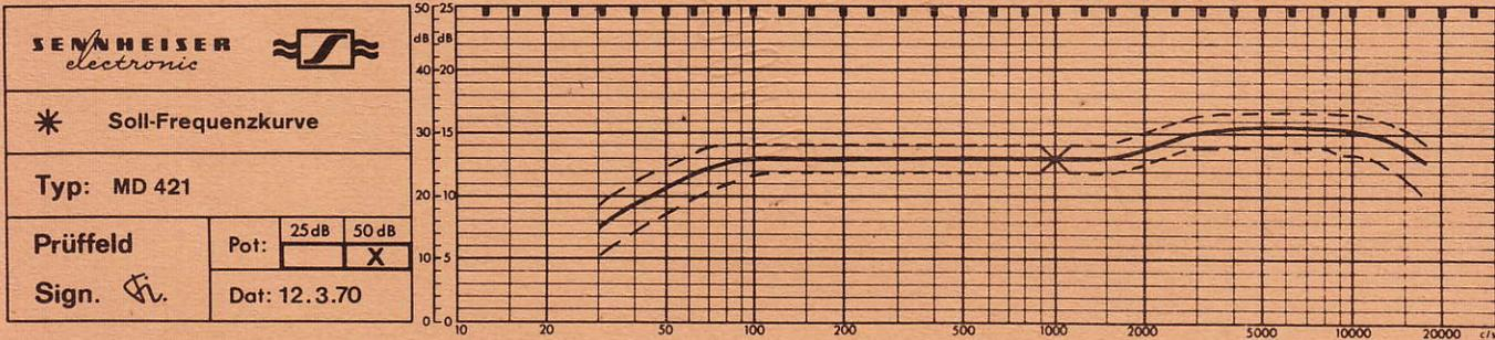
Nominal frequency response curve (with tolerance limits) MD 421
