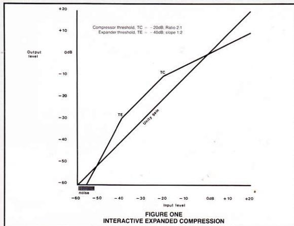
The example given is typical of cassette or cart program material being compressed for transfer or broadcast. As the program is compressed, the residual noise level is raised, in this case by 10 dB. The action of the expander reduces both the signal below the expand threshold, TE, and the residual noise as perceived at the output.
