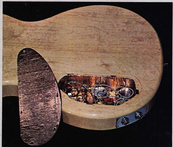
Every CARVIN guitar is completely shielded with heavy solid copper tape which totally surrounds the control area. Also, the pickup coils are shielded with copper tape, and the pickup wires are incased in a shielded jacket. The results are superior protection against hum or interference.
