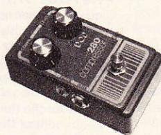
**Compressor 280** Here's a distortion-free sustaining unit that can be easily adjusted to compensate for your instrument's signal decay. If you increase the compression level, the Compressor 280 will make everything you play come out at a constant, pre-set volume. Decreasing the compression effect makes the unit a peak-limiting device that limits the maximum available output. Also features battery/AC battery eliminator operation.
