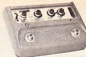
**Boss Chorus Ensemble CE-1** The Roland Boss Chorus combines vibrato and chorus effects in a sturdy, compact unit. Controls include a high/low input, output level, mono/stereo, chorus intensity, vibrato depth and intensity. Dual foot-switches enable the user to cancel or change effects as he sees fit. This is a great effect for both combo and solo performances, as it will really thicken up your sound.
