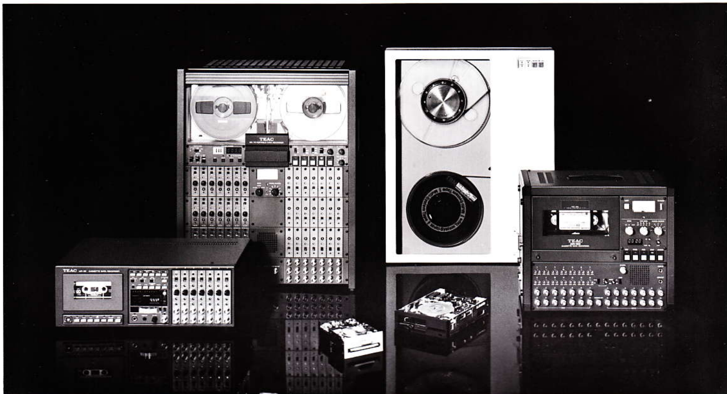
TASCAM Series 40 tape machines draw on TEAC's broad experience in storage technology: MR-30 7-channel portable cassette data recorder, SR-70 21-channel 1/2" reel-to-reel data recorder, MT-1000 1/2" digital memory system, XR-50 14-channel portable data recorder, FD-30A 3" 250 kilobyte compact floppy disk drive and FD-55 5-1/4" 1.6 megabyte mini floppy disk drive.
