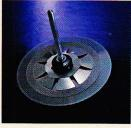
spaced, photo-etched radii, on the other hand, produces 15,000 pulses per second as the capstan rotates. By comparing the counted pulse-rate against a fixed reference, instantaneous speed-correction signals can be applied to the capstan within microseconds, helping lower the wow and flutter to a mere 0.035% WRMS.
