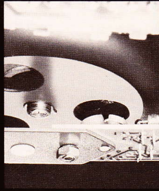
A motion sensor which reports the tape transport status to the control system is mounted underneath the right hand side tape drive motor.
