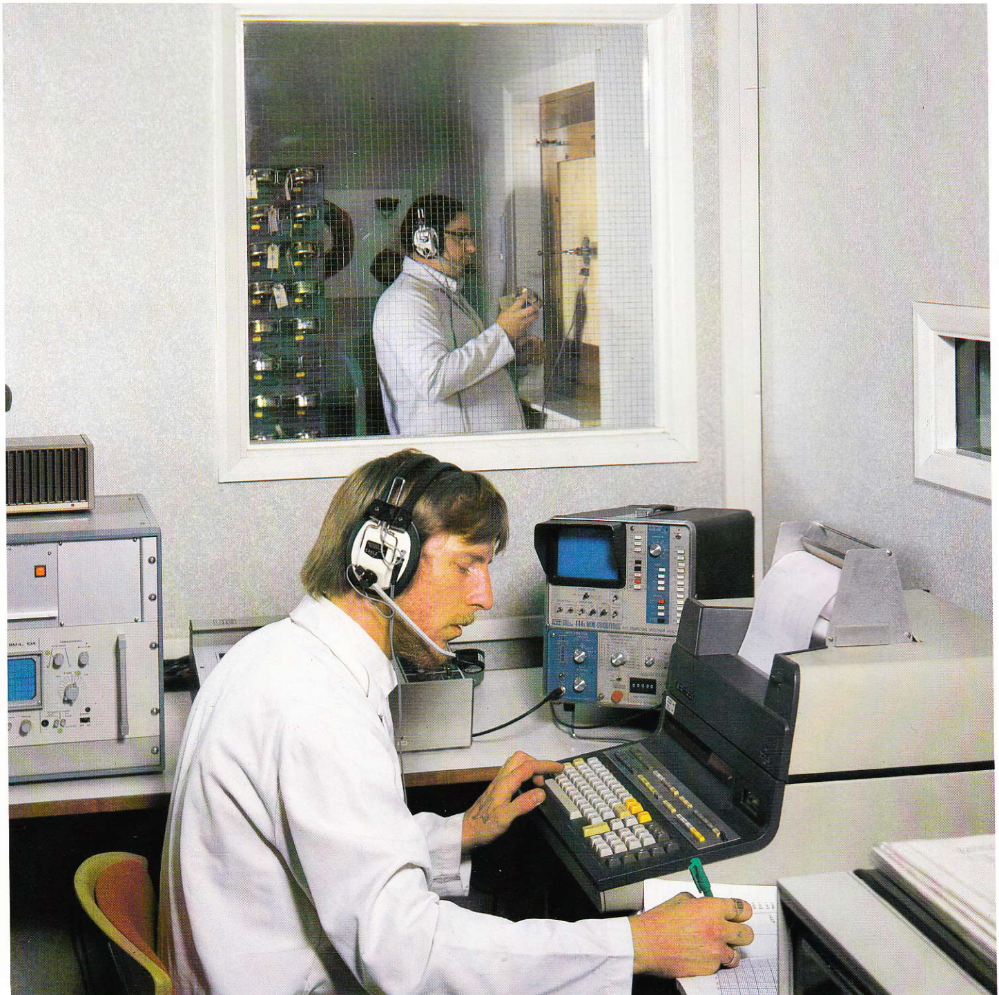
Drive units for every pair of Model 101 loudspeakers are selected and matched by computerised digital testing equipment to ensure that each pair of systems will perform to the same high standards as the prototypes.
