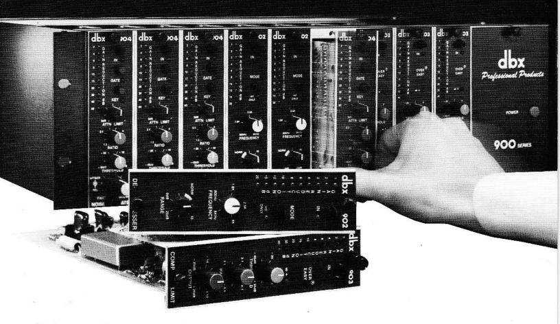
Today signal processing plays a greater role in sound production than ever before, both in the studio and on the road. As a result, rack space is at a premium. Innovative packaging eliminates redundant power supplies, simplifies interconnects, and saves space. With this in mind, dbx has created the 900 Series Modular Signal Processing System.
