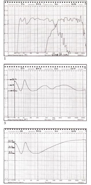
5 LF unit in external (Bi-amp) mode. Modulus of impedance using constant current source.
