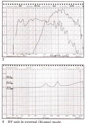
HF unit in external (Bi-amp) mode. Modulus of impedance using constant current source.
