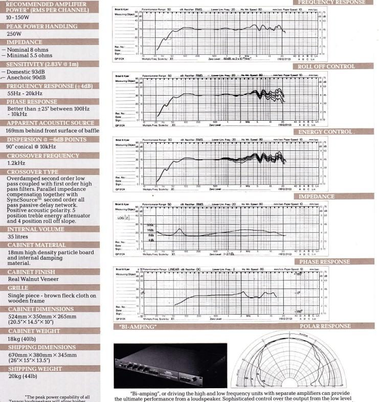
\*The peak power capability of all Tannoy loudspeakers will allow higher amplifier powers to be used with wide dynamic range material. Care must be taken owever, to avoid conditions such as switch on surges and amplifier overloading or 'clipping' which may result in momentary peaks of power greatly in excess of the specified ratings.
