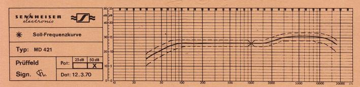
Nominal frequency response curve (with tolerance limits) MD 421. Every MD 421 is supplied with its own factory frequency response curve.
