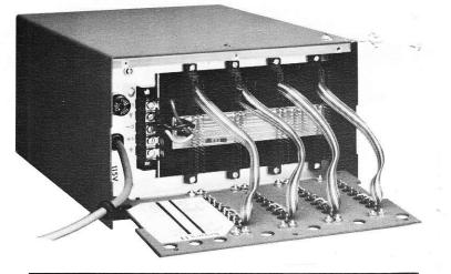
Audio interface is quick and simple through back panel mounted barrier strips. A hinged back panel allows access to the various accessory connections at the back of each card.
