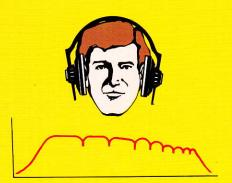
An **open air headphone** may also produce a similarly "measured" flat frequency response as the loudspeaker; however, air escaping around the ears weakens the effective bass response, while the earpads damp the desirable comb filter notches, again restricting perceived "normal" hearing.
