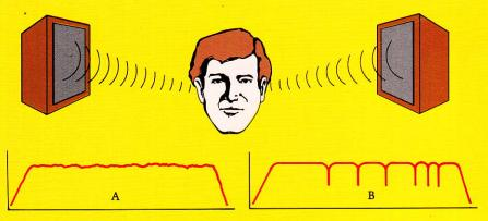
Loudspeakers yield a reasonably flat frequency response when measured in an anechoic chamber (A). Our ears and brain, influenced by their inherent comb filter (B), perceive the sound as ''normal'' and ''flat''.
