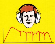
When "measured," a sealed headphone may produce a similar or better frequency response than a high-quality loudspeaker [A]. However, when worn, its tight seal around the ears exaggerates the bass response; while the location, number, and depth of the comb filter's notches are also severely altered, destroying the impression of "normal," flat sound.
