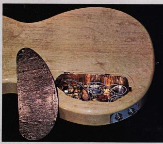
Every CARVIN guitar is completely shielded with heavy solid copper tape which totally surrounds the control area. Also, the pickup coils are shielded with copper tape, and the pickup wires are incased in a shielded jacket. The results are superior protection against hum or interference.
