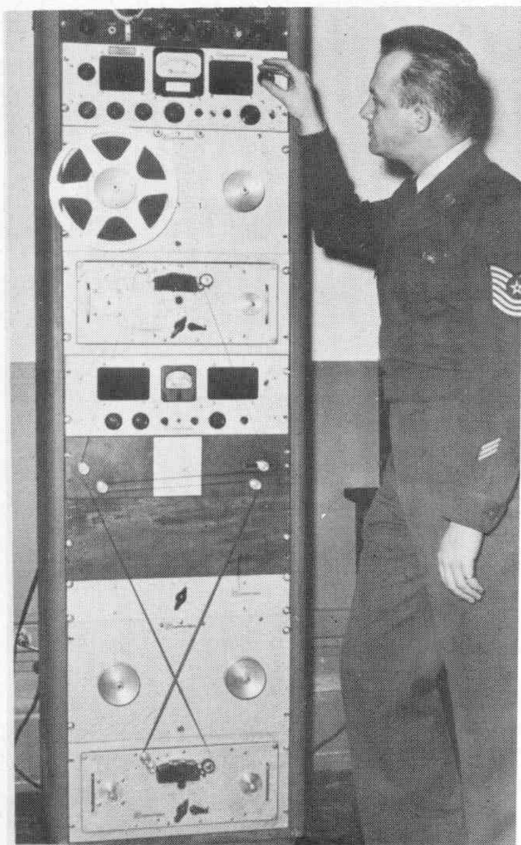
Recorder setup for the time-delay loop showing the two Magneorders, special panel with insion roller and ampliér which form the basis of method described by Lt. Jesse C. Durham, USNR, for AFRS "Editing without Cutting Tape."
