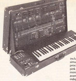
ARP 2600 (duophonic) The 2600 might best be viewed as a portable studio synthesizer for live, educational and recording use. The front features Arp's linear slider mixing approach, however all hard-wired signal routings can be over-ridden via patch cords and patch points on all functions. Other features
