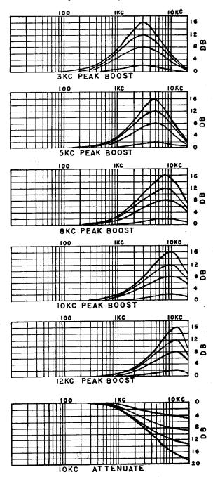
The boost and attenuate controls are continuously variable. Therefore, the curves in the above families represent typical settings, not steps.
