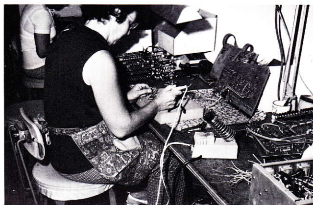
In this group, various stages of component assembly are seen. The skilled women workers handle a large part of the individual assembly, rather than strictly working on a pass-along basis—though this technique is also used.
