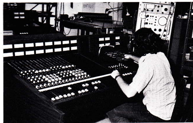
In these two photographs the console construction area is shown. Gately makes even the cabinets in his woodworking shop. With modules and components inserted, each console is given a painstaking shakedown before it goes out the door. We were told that it takes an average of seven men working one month to create a finished console.
