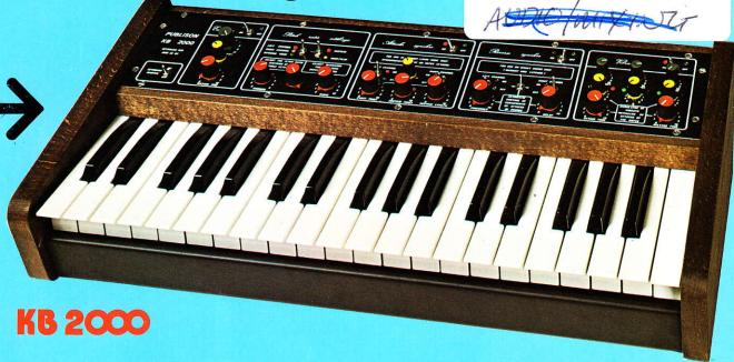
KB 2000 is an external programmation unit for the audio computer DHM 8 9 B2. It includes a three octaves piano keyboard, and a control panel for setting the following functions:
