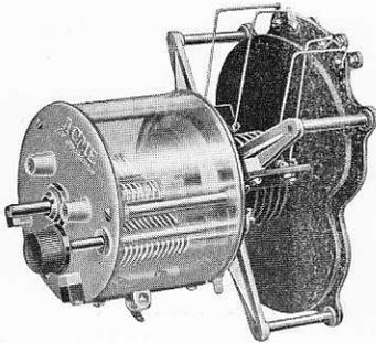
Tuned radio frequency amplification gives greater distance and selectivity when used with Reflex. In order to keep tuning control to a single unit and increase efficiency the Acme Apparatus Co. developed the "D" Coil Unit which consists of a tuned R.F. transformer mounted on the shaft of an Acme low loss condenser so that it can be tuned simultaneously with the loop circuit. The coil is mounted on bakelite moulded forms and is extremely low in R.F. resistance.
