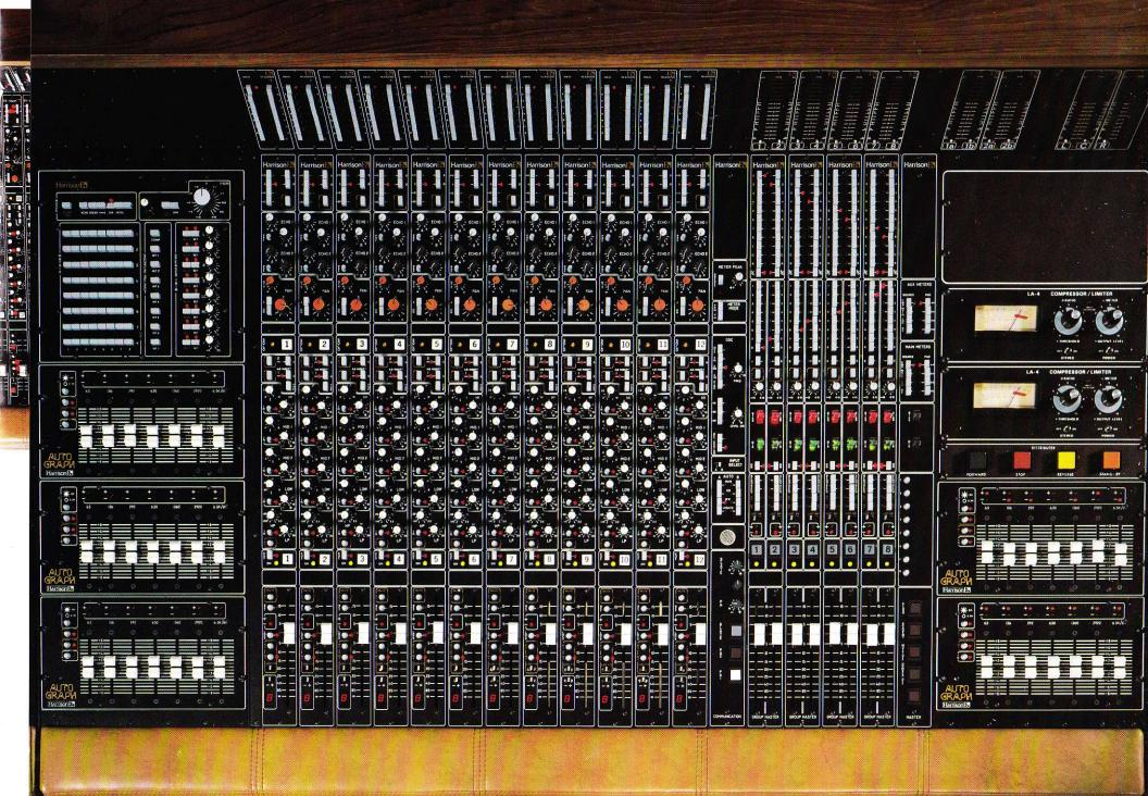
A major development is the concept of "Distributed Control Intelligence" (DCI). This involves placing an individual microcomputer in each input module of the console. This "DCI" concept offers the end-user many advantages over the older 'hardware logic controlled' analog consoles. Included in these advantages are tremendously expanded automation opportunities, improved ergonomics (human engineering), better reliability, easier maintenance, and many side benefits such as noiseless switching.
