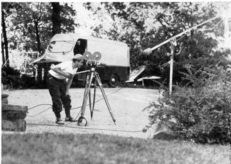
C. Robert Fine, designer and builder of the "location" unit, is shown using the synchronous 16mm magazine loading Maurer camera which is being used for color work. A Telefunken microphone is at the end of the boom. The microphone and camera are equipped with 200' of extension cables. Since the recording truck can operate 600' from the generator trailer, it is thus possible for the microphone to be as far as 800' from the generator. This is quite useful for work done in the narrow winding streets which are characteristic of numerous historical European towns and villages. Remote controls enable one man to operate all equipment that is inside the truck while he is at the camera or microphone boom.
