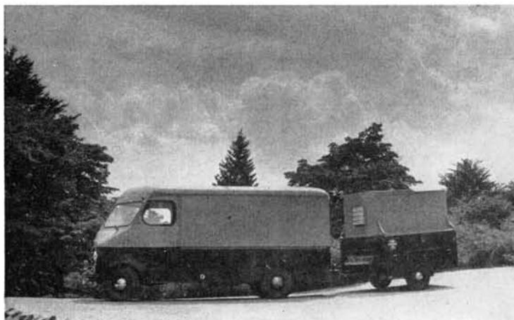
The "location" unit (it hasn't been christened with a name as yet) consists of a 1-ton, 6-cylinder Chevrolet truck with an aluminum body. It is equipped with an extra gas tank to take care of those long stretches between European re-fuelling stations. All of the operating equipment is contained inside the truck which has sufficient space for two operators to move about without crowding or stooping. There is adequate floor space for sleeping cots, in case of emergencies.
