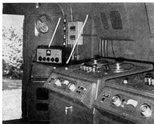
The two racks of equipment shown in the block diagram are mounted against the bulkhead opposite the Magnecord mixer location. The racks are hinged at the bottom and secured at the top with wing nuts and bolts so that they can be made to swing forward and rest against the restraining chains, exposing their interiors for service and inspection.
