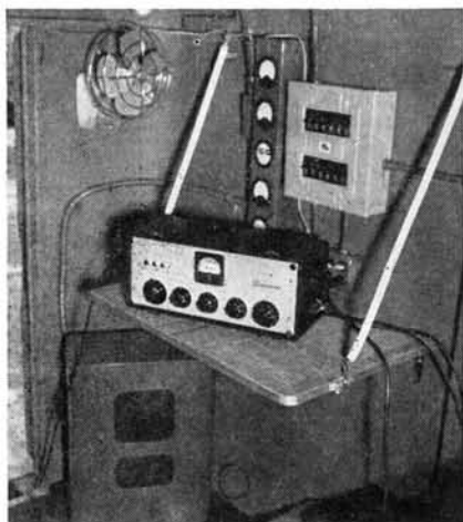
The microphone and audio mixer is a Magnecord PT6-P. It can be operated inside or outside the truck. Below the Magnecord mixer can be seen a small Jensen bass-reflex baffle equipped with long extension lines so that it can be placed near the subject being photographed.
