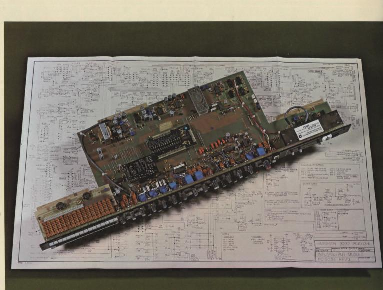
The stereo cue send system on each I/O module consists of a level pot, a stereo pan pot, and a "PRE/POST" switch. The PRE and POST inputs to the cue come individually from the FET switching card.
