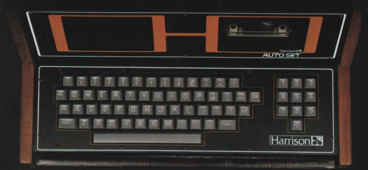
AUTO-SET is not a single piece of equipment. Rather it is a system of process control micro-computers designed for the entertainment industry, and manufactured by Harrison Systems.
