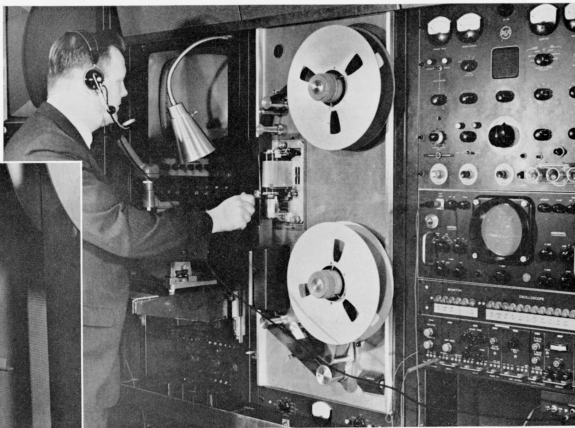
FIG. 16. View of air bearing head-wheel showing Ed Welsh adjusting head for no scalloping during playback, using a special tool built at Reeves.
