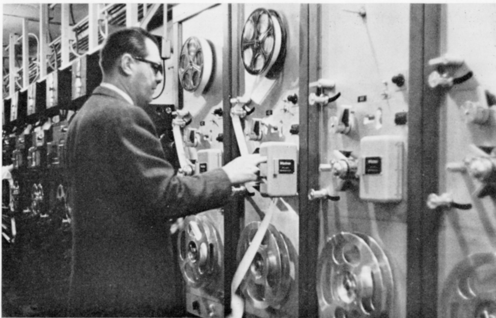
FIG. 13. Sound dubber room, showing several of 40 sound playback machines, which use sprocketed magnetic or optical film. Richard Vorisek loading dubber.
