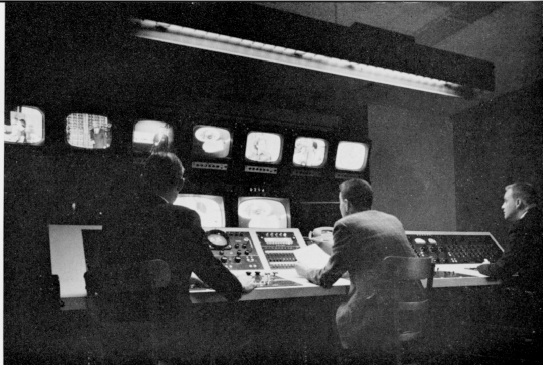
FIG. 8. Studio X—one of two mixing rooms showing input, preview and program monitors. The left side of the console is for video control, the right side for audio control. There are 9 video inputs, 18 audio channels. Dissolves and 150 RCA effects can be made here.
