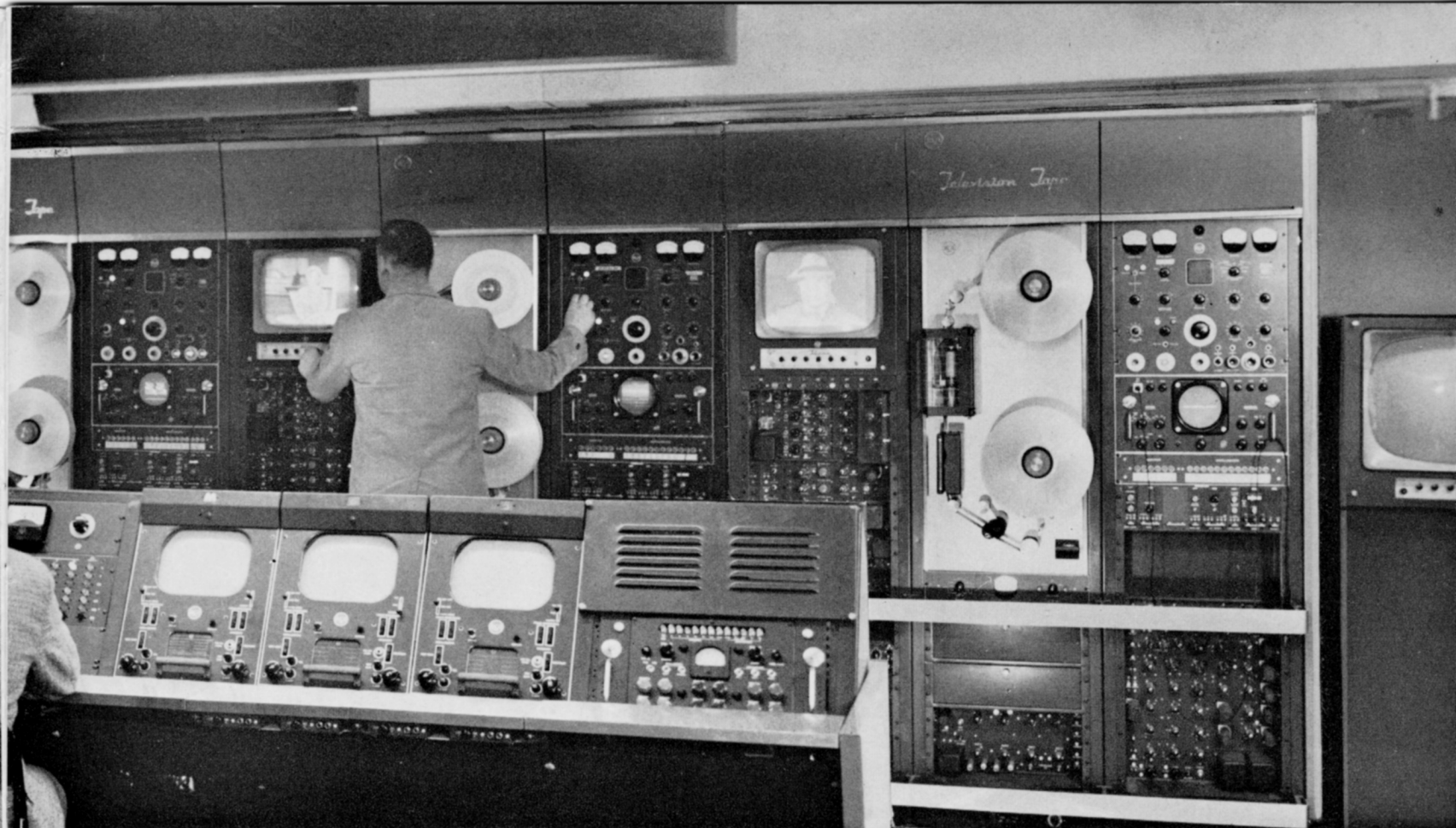
FIG. 1. Main Recording Room. This view shows six of the RCA television tape recorders and the camera control console.
