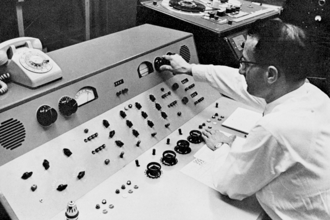
FIG. 3. Sound Transfer Console. All sound tracks going to film are equalized through this console.
