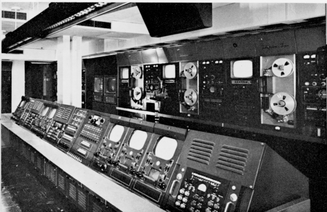
FIG. 9. The camera switching and central control position in the main recording room. From this position all equipments can be started and stopped, monitored and switched.
