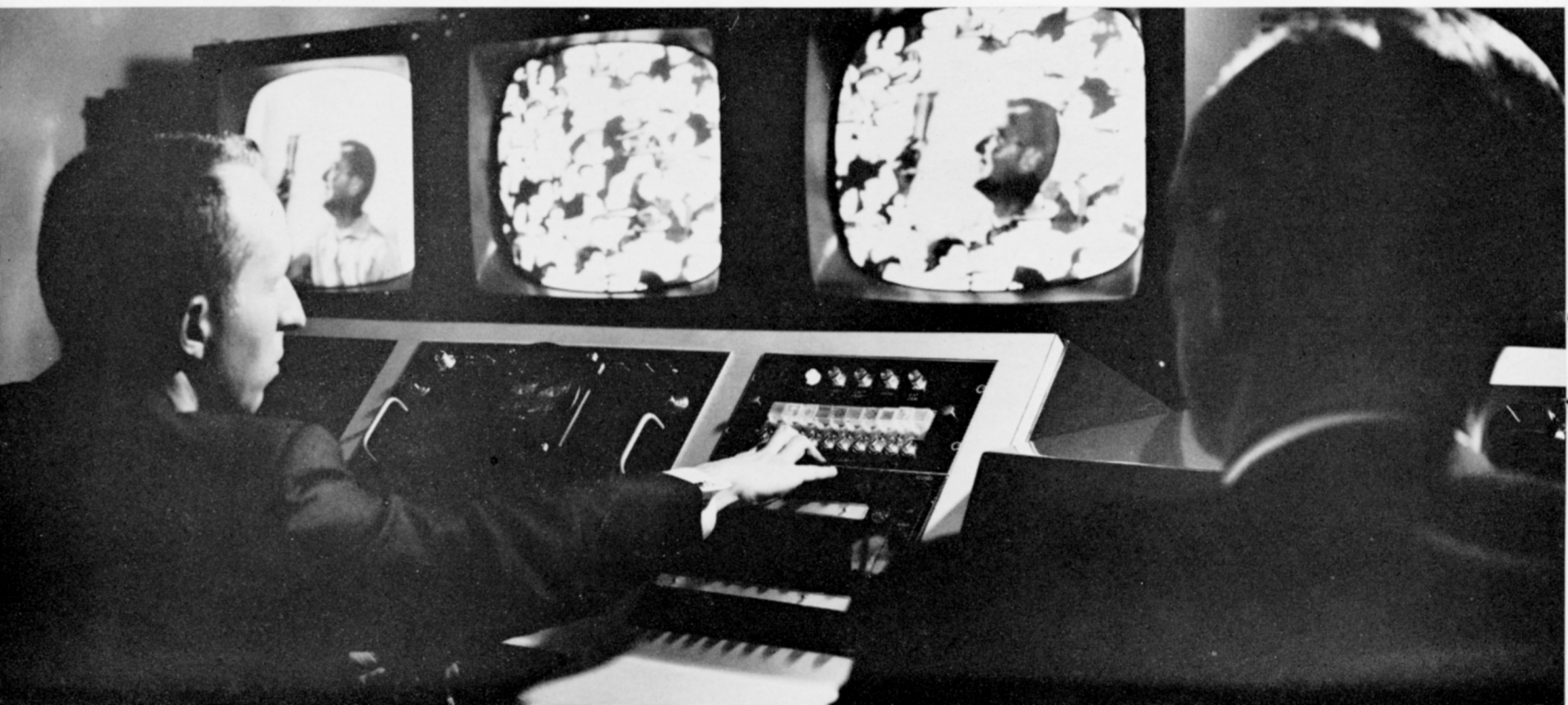
FIG. 28. The RCA special effects control panel in operation at Studio X. Note effects produced as shown on monitors.
