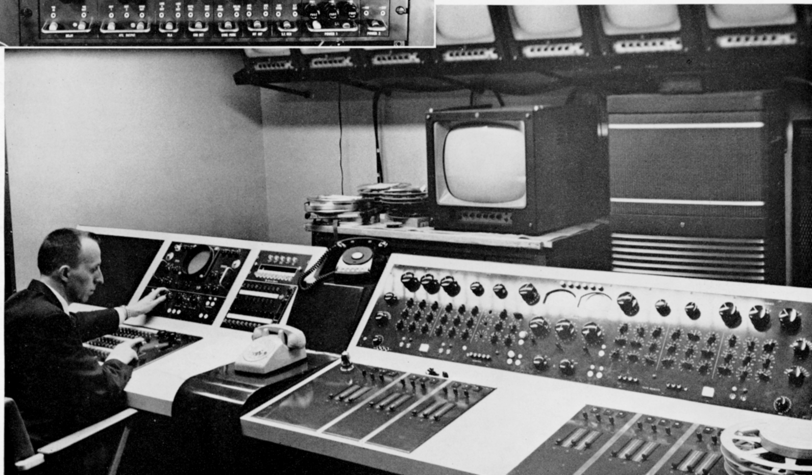
FIG. 22. Audio console (right) and video (left) of mixing studio Y, which is equipped identically to Studio X. Charles Power, maintenance engineer, is shown at TS-40 Transistorized Switcher panel.
