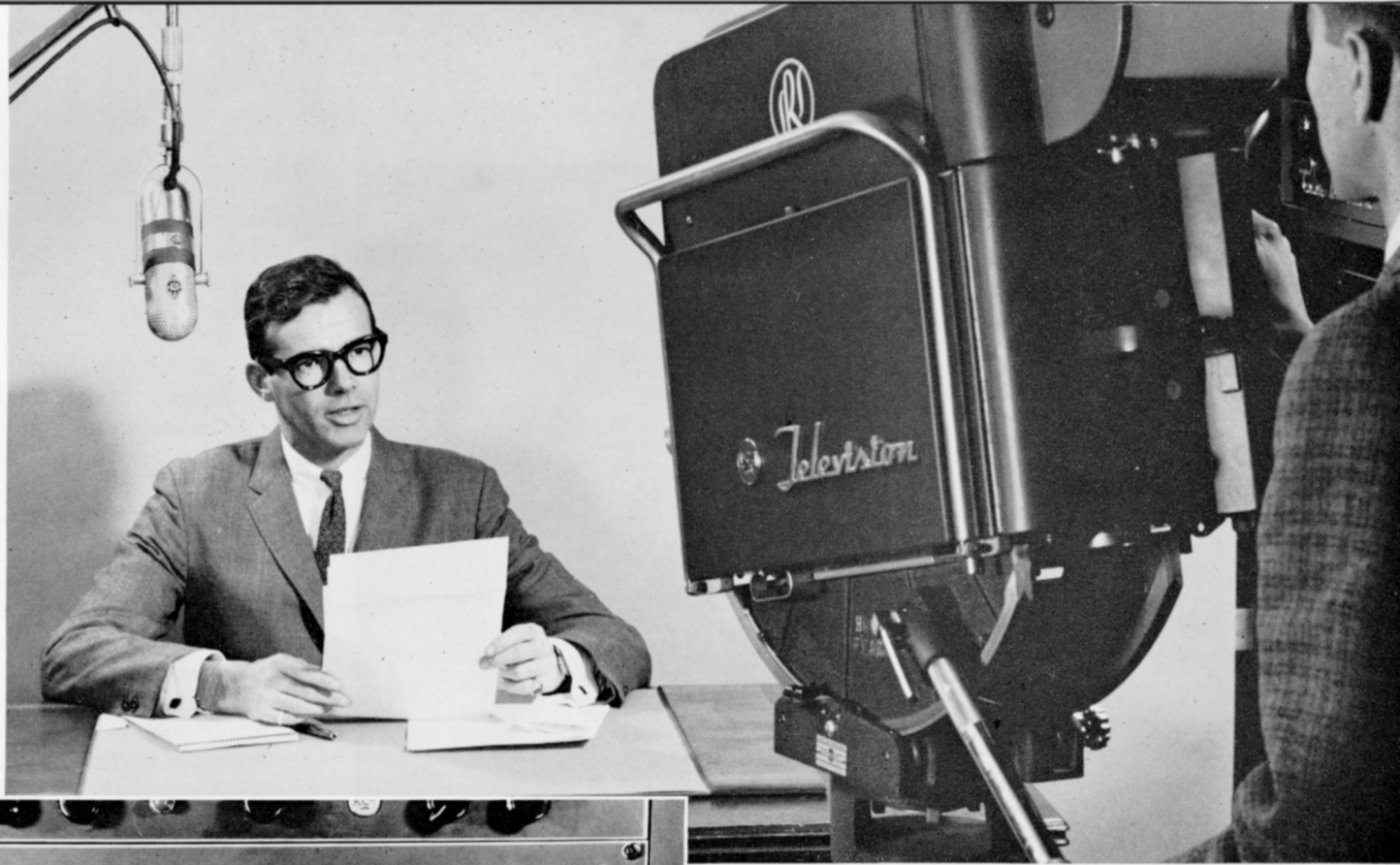
FIG. 20. Type TK-11 monochrome live camera at Reeves Studios is used for simple shots or commentary recordings in conjunction with location or studio recordings.
